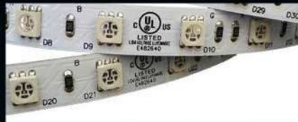
Cinta LED Flexible UL de 72W RGB (14.4W/m)
